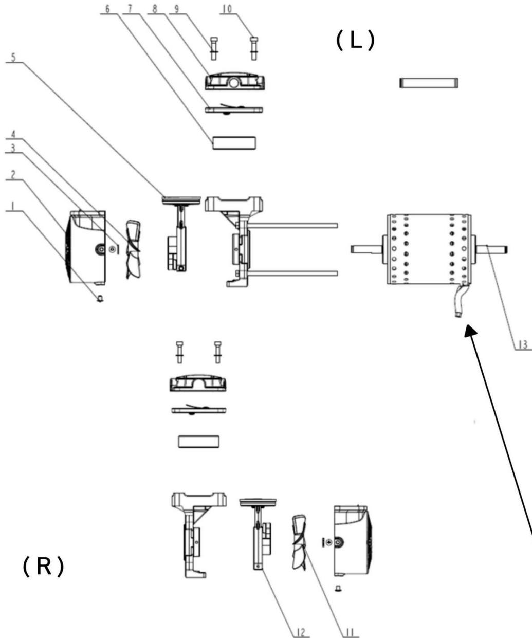
NOTE: Left and right side components are determined by viewing motor/pump from the back or with power cord coming out of lower right-hand side of motor.
